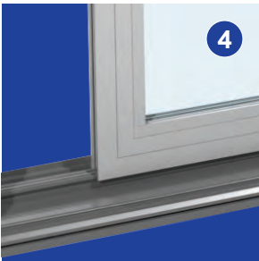
High water barrier bar at the sill to prevent water penetration.
